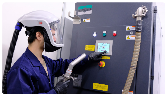
Russell AMPro® Sieve Station installation
