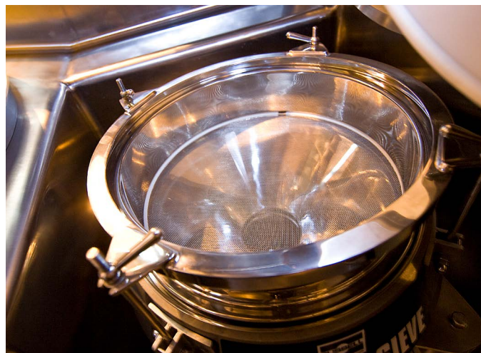
图3.全不锈钢Russell Compact Sieve®紧凑型振动筛
