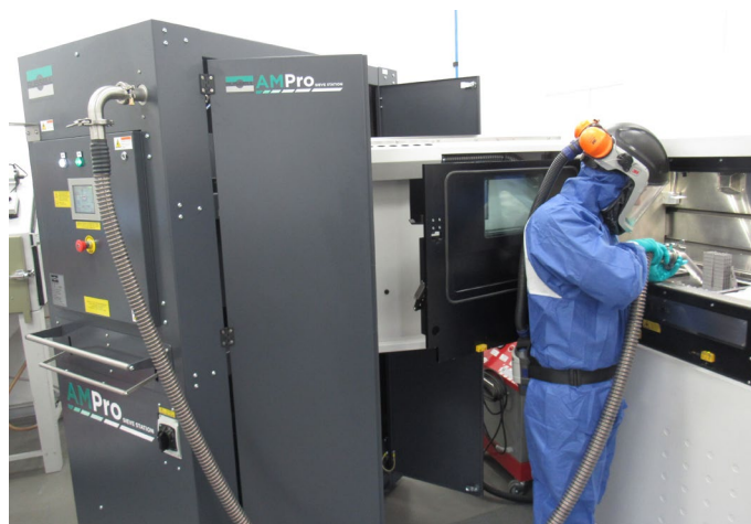
Figure 1. Progressive Technology 使用Russell AMPro Sieve Station™粉末筛分回收系统筛分回收AM增材粉末
